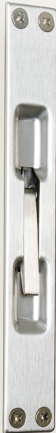
Manually switching the lever/snib upward for retracting the bolt to unlock the inactive leaf, and downward for projecting the bolt to lock the inactive leaf, all done while the active door is opened.
