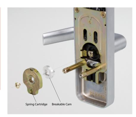
Model 508 Trim is composed of heavy duty investment cast steel. An internal breakable cam breaks away when a predetermined load is applied to the outside lever handle in locked mode without damaging the trim or compromising security. The cam is easily replaceable with minimum efforts.
