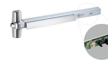
The Alarm Exit provides a simple way to audibly monitor the use of an exit device. The unit contains an alarm which is activated when the Push Bar is depressed. The alarm sounds at 85 db. The unit operates on one standard 9-volt alkaline battery. When the battery is weak, the horn will emit an intermittent low battery alert signal. Can also be powered using the PS100 series Power Supply.
