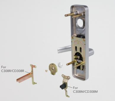
When locked, the lever handle will turn freely and disengage from the center case of the exit device. When an excessive force is applied on the lever handle, it will cause the breakable cam inside the trim to break at a predetermined load, protecting the trim from further damage.
