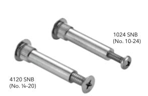
Furnished standard with machine screws. Specify sheet metal screws or wood screws when/if required. Specify Sex Bolts (SNB) where recommended or required by the door manufacturer.
