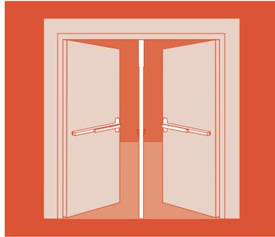
Removable mullions are used with paired doors where a full width opening is only occasionally required. Doors are fitted with Rim Exit Devices and normally function as single doors. Available in 7', 8' or 10' lengths.
