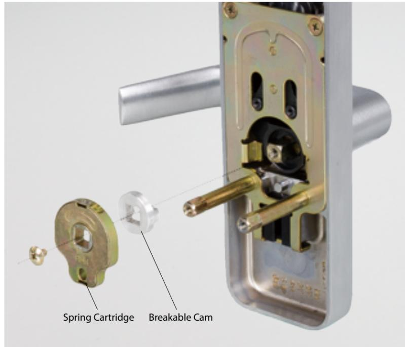
Model 308 Trim is composed of heavy duty investment cast steel. An internal breakable cam breaks away when a predetermined load is applied to the outside lever handle in locked mode without damaging the trim or compromising security. The cam is easily replaceable with minimum efforts. The spring cassette and the breakable cam are replaceable parts.
